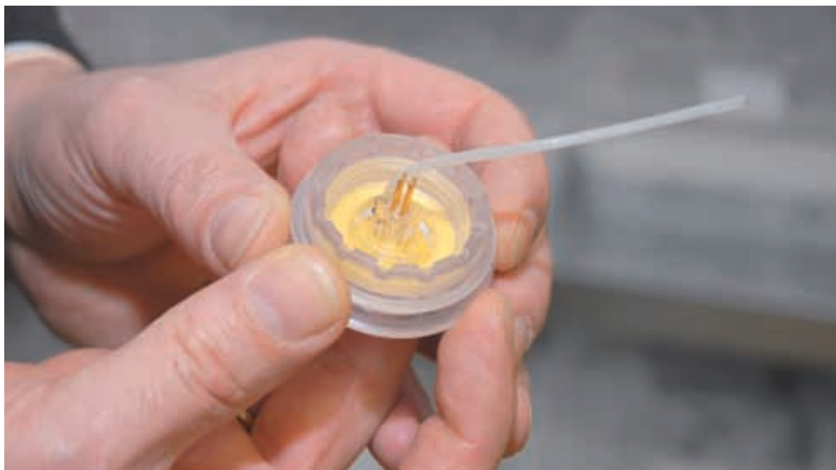
The silicon hose of the press key compensates for pressure fluctuations and protects against vandalism and malfunctions in the button
